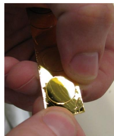
Figure 1: Peeling off glass cover slip to expose fresh gold surface.
