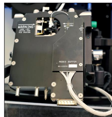
Figure 1: AFM Modes bottom board attached to the DPN 5000 system scanner.
