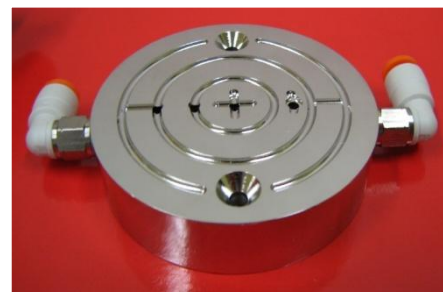
Figure 1: Vacuum Sample Stage for holding substrates and inkwell arrays on the DPN 5000 System.
