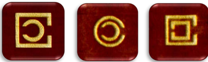
Figure 1. Gold nanostructures fabricated on silicon surface. The structures have a line width of 400nm and a height of 12 nm.
