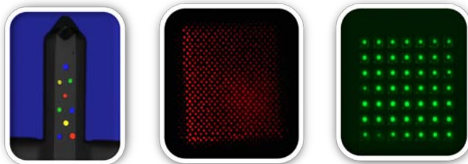
Figure 2. Fluorescent images of protein printed on microfabricated structures. The image on the left is that of an AFM cantilever with four different proteins. The middle and right images are of polymer pillars with fluorescent proteins printed on them. The pillars in the middle image are 1.5 microns in diameter while those in the right image are 10 microns square.
