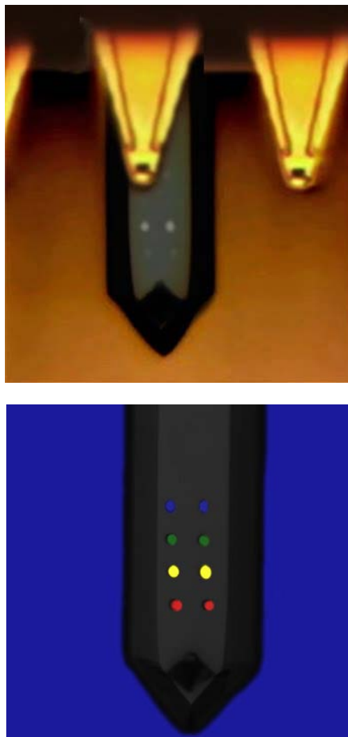
Figure 1. (Top) Brightfield live image showing the printing of 6-micron dots of fluorescently tagged IgG onto a commercially available AFM cantilever. (Bottom) Fluorescent image of the printed domains on the cantilever.
