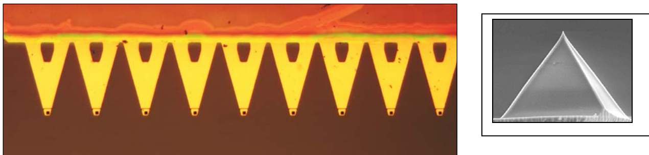
Figure 3: An optical microscope image and expanded area of the inkwell.
